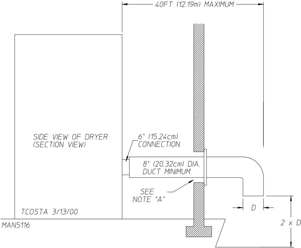
NOTE A: OPENING MUST BE 2-INCHES (5.08cm) LARGER THAN THE DUCT (ALL THE WAY AROUND). THE DUCT MUST BE CENTERED WITHIN THIS OPENING.
