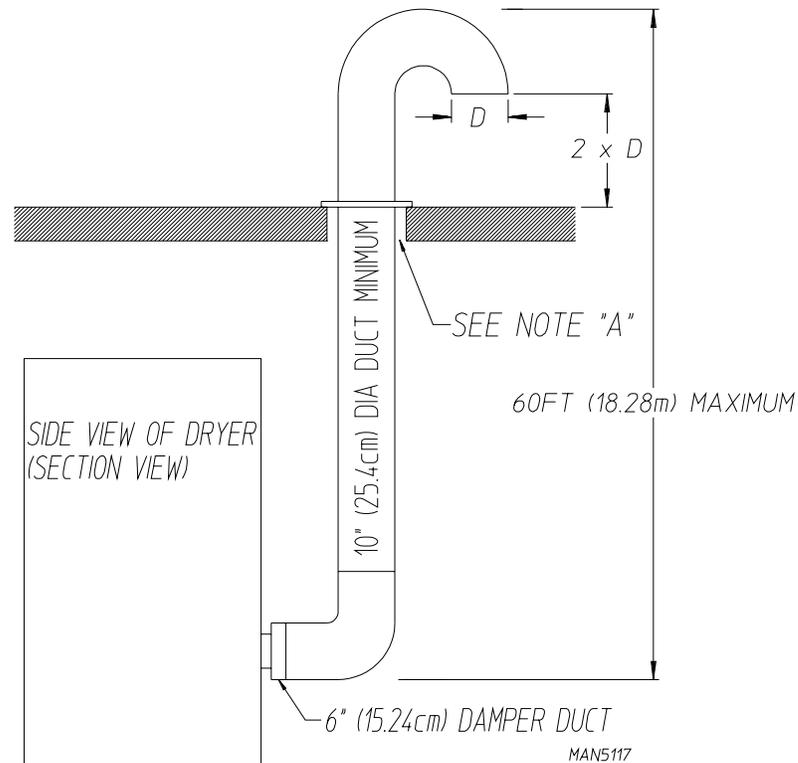
NOTE A: OPENING MUST BE 2-INCHES (5.08cm) LARGER THAN THE DUCT (ALL THE WAY AROUND). THE DUCT MUST BE CENTERED WITHIN THIS OPENING.
